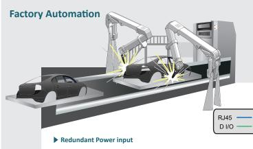
The Woodpecker 8015 Series has dual power inputs to provide a redundant system against power supply disruptions. In case of one power source failure, the other acts as a backup to remain continuous network power for critical industrial applications.
