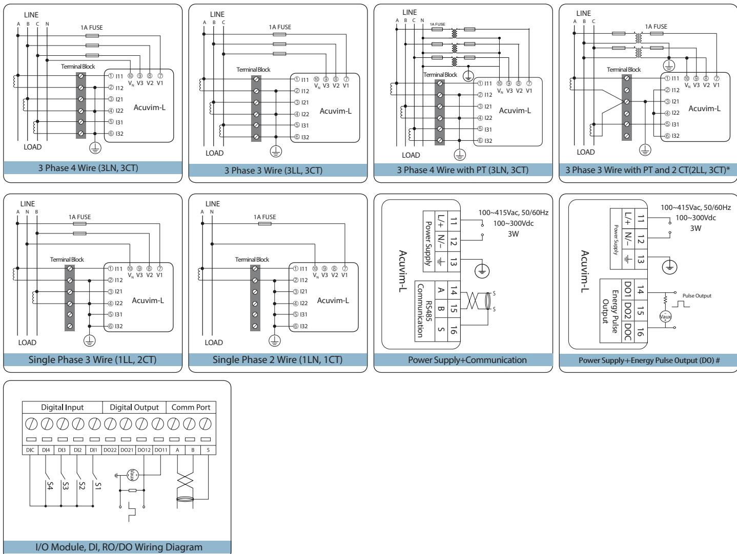
Note: 1. \*\*\* 2CT configuration is optional only in 3 Phase 3 Wire system; 2. # Wiring diagram is only applicable to Acuvim BL.
